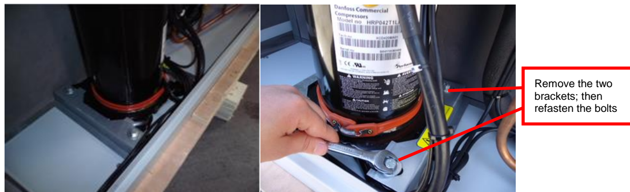
Figure 11: Remove Compressor Brackets
