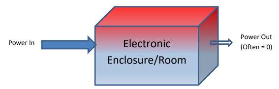
**NOTE:** If the equipment is powered from a DC plant, the heat generated from rectifier loss should be added to the electronics heat load.
