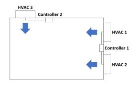
**Solution:** Since each controller controls one or two HVAC units, these 3 units require 2 controllers. For reference, let HVAC 1 and HVAC 2 connect to controller 1 and HVAC 3 connect to Controller 2.
